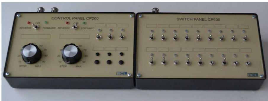
The Switch boards and indicators come in 3 types. All types have screw terminals to connect the switch and the LED, (no need for soldering in a tight space.) as they come pre assembled on a printed circuit board. Installing them into the panel only requires the fixing of the switch in place, the LED is at a preset height so protrudes through the second hole to the right height.
